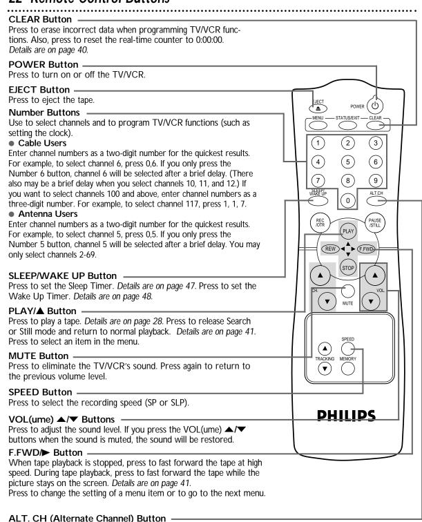
Press to return to the TV channel you were viewing immediately before switching to your current channel.
